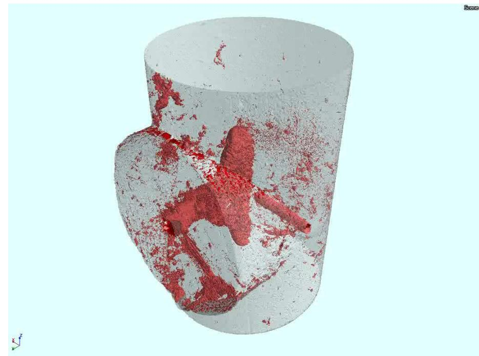
Hot tear and porosity in Al-casting
